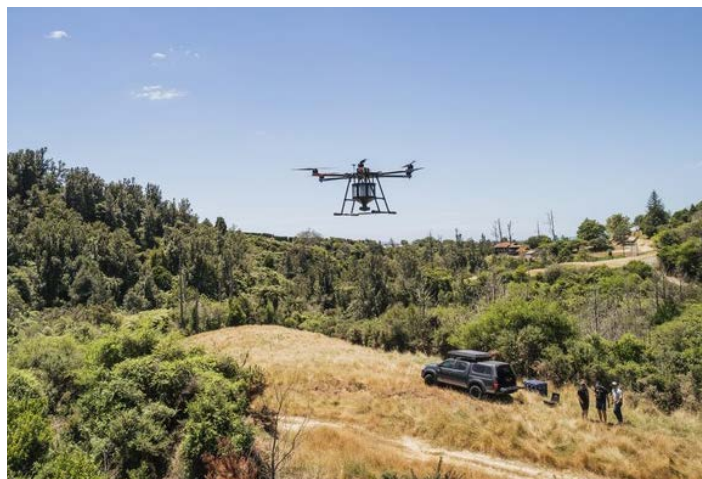
An Envico-developed UAV with a 20kg bait applicator being flown over farmland and native forest in the western Bay of Plenty. Photo: Envico
