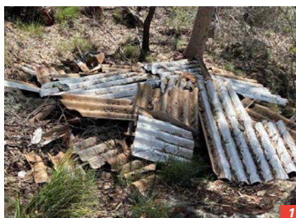
1/ Some of the dumped asbestos panels had been painted green.
