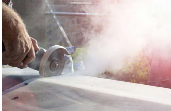
The engineered stone ban came in response to risks to workers from dust caused by cutting, drilling, polishing and more. Photo: courtesy WeAre.SA
