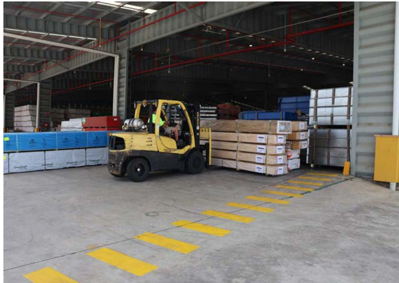
Clearly marked walkways for pedestrians are vital, particularly in zones where forklifts operate. Image: Campbell McInnes
