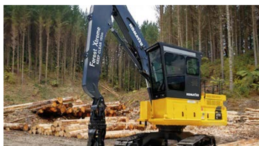
The Komatsu PC270LL-8 is the smallest of the Log Loading Xtreme Carriers and is fitted with the Osaka factory High Wide Undercarriage. Photo: Komatsu
